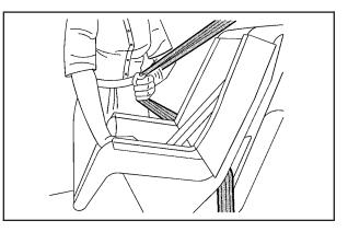
4. Pull the rest of the shoulder belt all the way out of the retractor to set the lock.
